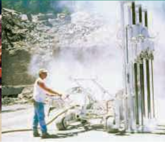
A-3SD Vertical Quarry drill with a 3658mm drill depth.
