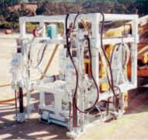
A-4SD Vertical Equipment mounted drill that can drill in five different configurations.
